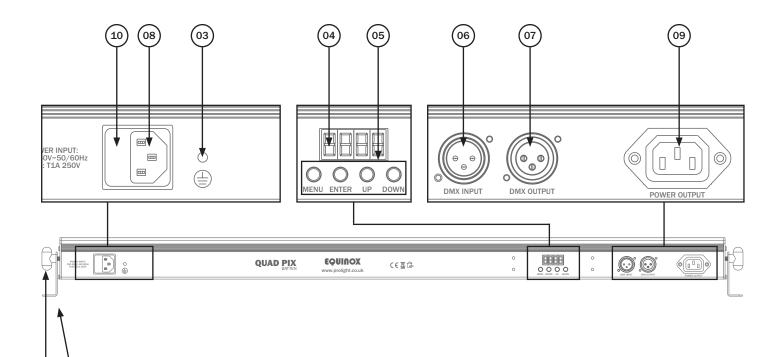
01 - Bracket tightening knobs05 - Function buttons02 - Bracket06 - 3-Pin XLR input03 - Earth point07 - 3-Pin XLR output04 - LED display08 - IEC power input
